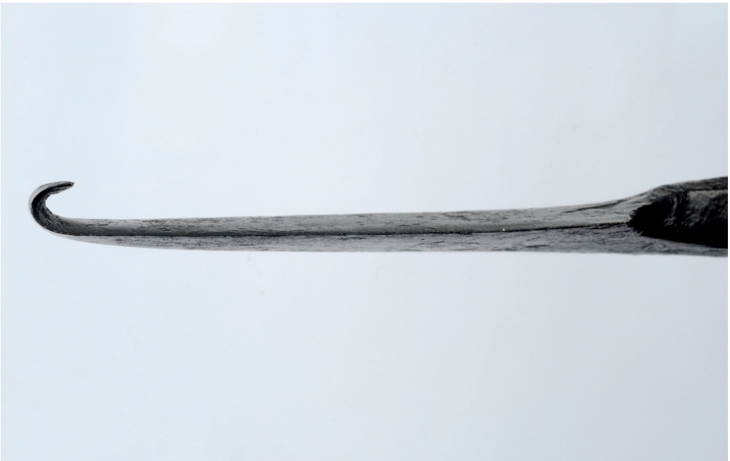
Fig. 3. Groove plane from Elbląg, detail 2. Visible are the hooked endings of the arm of the tool and the line of the edge. Photo: M. Dąbski.
