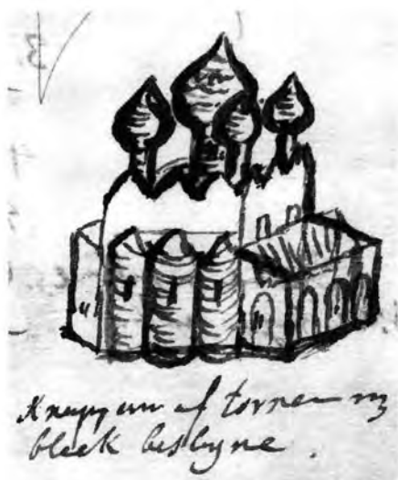
Fig. 8. knopparna af tornen m3 bleck beslagne. — the knobs of the towers are covered with tin-plate
